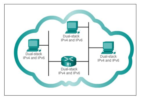
Dual-stack: Allows IPv4 and IPv6 to coexist on the same network. Devices run both IPv4 and IPv6 protocol stacks simultaneously.
