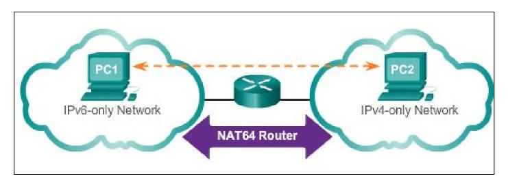
Translation: The Network Address Translation 64 (NAT64) allows IPv6-enabled devices to communicate with IPv4-enabled devices using a translation technique similar to NAT for IPv4. An IPv6 packet is translated to an IPv4 packet, and vice versa.
