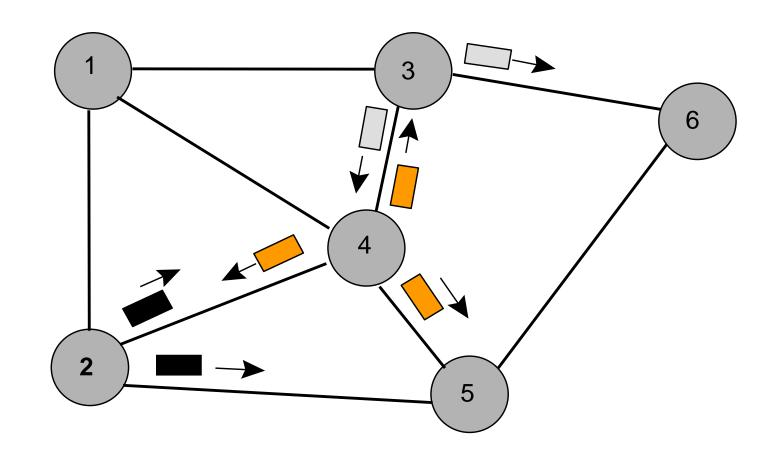
Flooding is initiated from Node 1: Hop 2 transmissions
