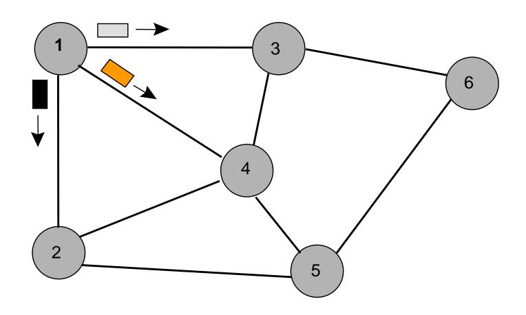
Flooding is initiated from Node 1: Hop 1 transmissions
