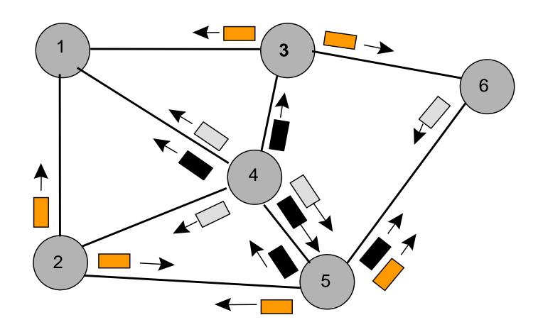
Flooding is initiated from Node 1: Hop 3 transmissions
