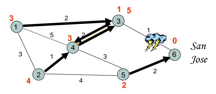
Network disconnected; Loop created between nodes 3 and 4
