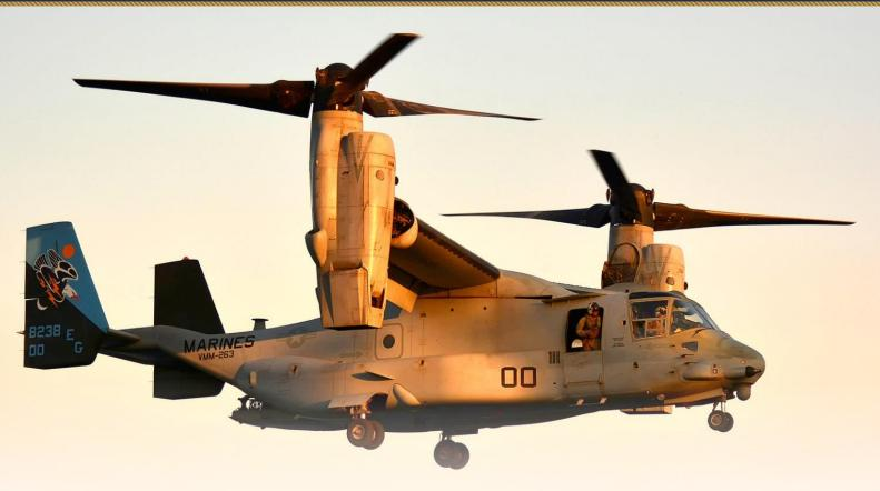
The MV-22B Osprey is a tiltrotor V/STOL aircraft that can operate as a helicopter or a turboprop aircraft and offers twice the speed, six times the range, and three times the payload of the CH-46E helicopter.
