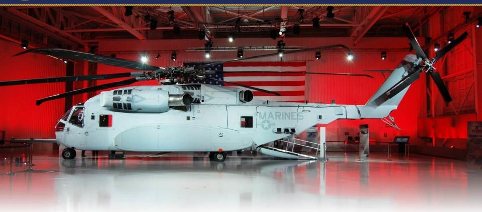
The most powerful helicopter in the Department of Defense, the CH-53K is a new-build helicopter that will expand the fleet's ability to move more material, more rapidly. Designed to lift nearly 14 tons at a mission radius of 110 nautical miles.
