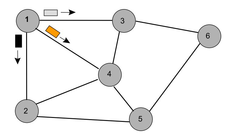
Flooding is initiated from Node 1: Hop 1 transmissions
