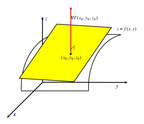
Recall that to write equation of a plane, we need a point on the plane and a normal vector. Since  $\nabla F(x_0, y_0, z_0) = \langle F_x(x_0, y_0, z_0), F_y(x_0, y_0, z_0), F_z(x_0, y_0, z_0) \rangle$  represents a normal vector to the surface (and the tangent plane), its components can be used to write the equation of the tangent plane at the point  $(x_0, y_0, z_0)$ . The equation of the tangent plane is given as follows:
