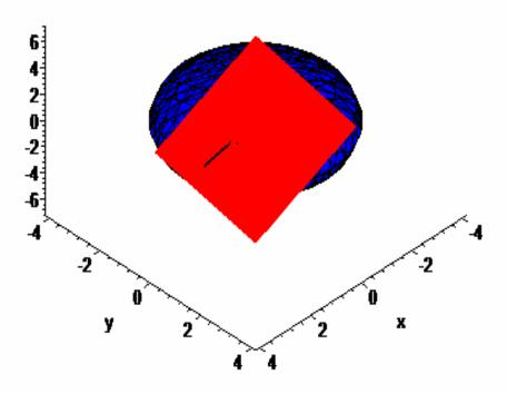
**Example 8:** Find the equation of the tangent plane and the parametric and symmetric equations for the normal line to the surface  $f(x, y) = e^{-x^2 - y^2}$  at the point  $(0,1,\frac{1}{\rho})$ .
