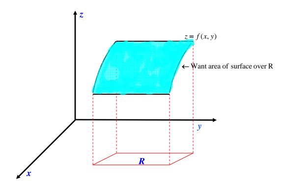
This surface area can be calculated using the following double integral.
